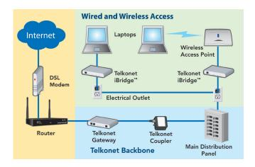
Telkonet's iWire System enables broadband access over electrical wiring, converting power outlets into high-speed data networks.
