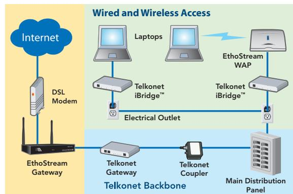
The Telkonet iWire System™ provides both wired and wireless connectivity, with Internet access at every electrical outlet.
