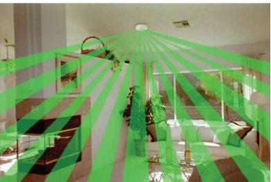
These diagrams illustrate the coverage pattern of the SS2000 Occupancy Sensor, showing how an entire room is scanned for motion.
