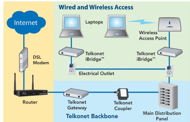
Telkonet's iWire System enables broadband access over electrical wiring, converting power outlets into high-speed data networks.
